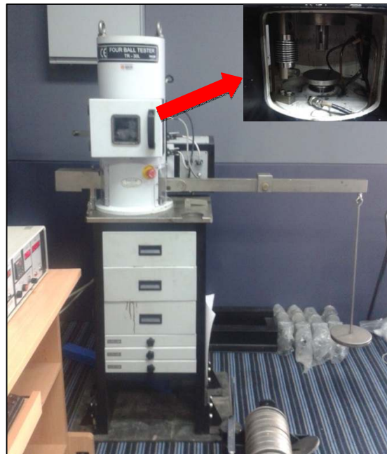
Figure 1: Photograph of a four-ball tribotester machine. The standard balls used in this experiment are made from AISI E-52100 chrome alloy steel, with the following specifications: diameter 12.7 mm; extra polish (EP) grade 25; hardness 64–66 HRC (Rockwell C Hardness). Four new balls were used for each test. Each time before starting a new test, the balls were cleaned with acetone and wiped dry using a fresh lint-free industrial wipe.
