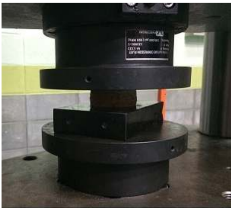
Figure 2: Test of compressive strength using Instron machine
