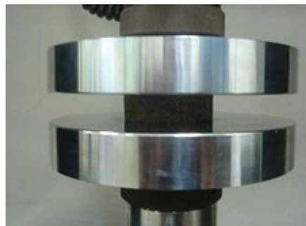
Figure 2. Briquette Undergoes Compression Test
