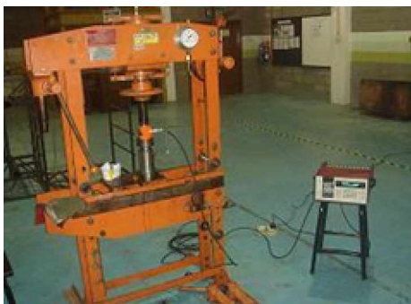
Figure 1: Experimental Setup for Briquetting
