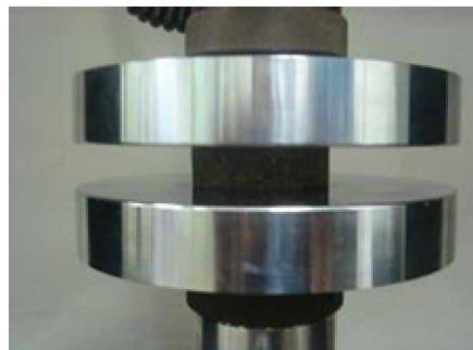
Figure 2. Briquette Undergoes Compression Test
