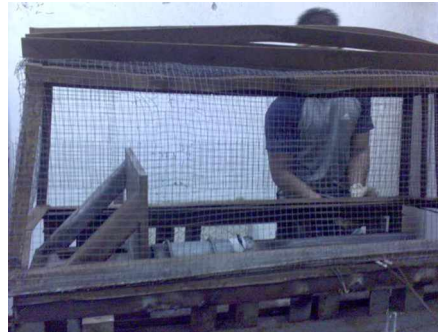
Figure 4.2: Caging of the rocket motor
